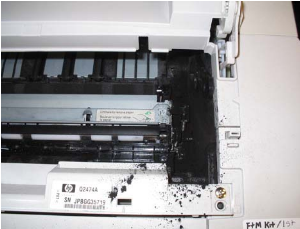
Brand F – Premature Failure leaking toner into the printer.
