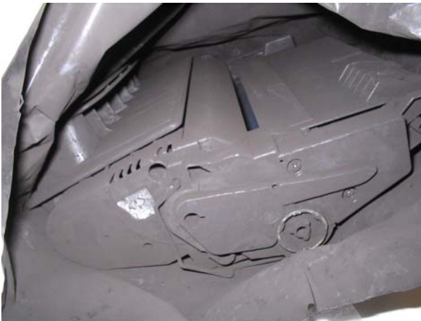
Brand I – Dead on Arrival – severe toner leak in the packaging.
