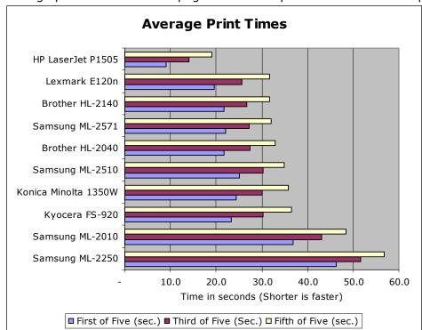
The following table shows the printers tested, their manufacturer specified print speed for letter size paper and first page out times, if available, compared to the actual performance achieved during testing by QualityLogic.
