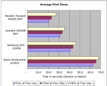
The following table shows the devices tested, their manufacturer-specified print speed for letter size paper and first page out times, if available, compared to the actual performance achieved during testing by QualityLogic.
