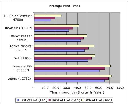
The following table shows the printers tested, their manufacturer-specified print speed for letter size paper and first page out times, if available, compared to the actual performance achieved during testing by QualityLogic.
