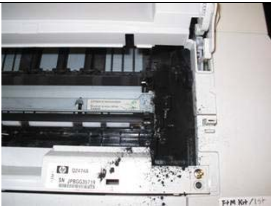
Brand N – Premature Failure leaking toner into the printer.
