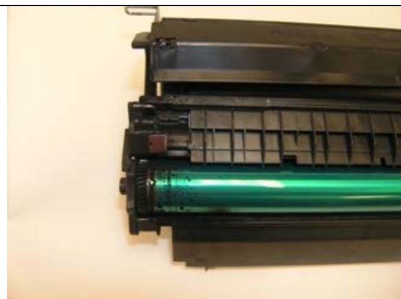
Brand G – Premature Failure cartridge leaking toner.
