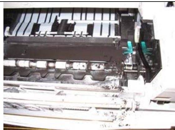
Brand M – Premature Failure leaking toner into the printer.
