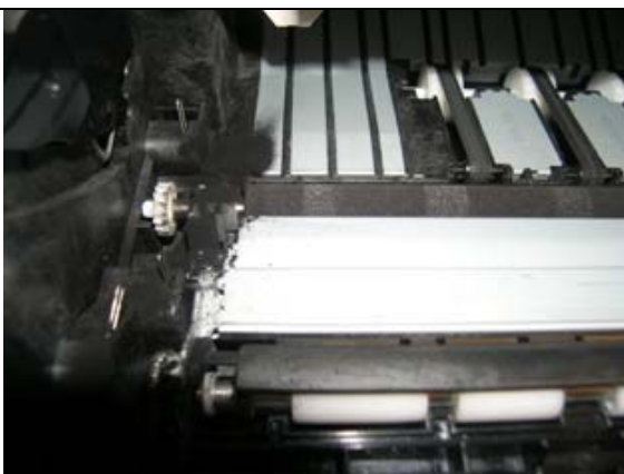
Brand G – Premature Failure leaking toner into the printer.
