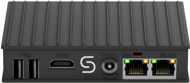
SwitchDIn Droplets with IEEE 2030.5 client act as secure gateway devices (SGDs)
