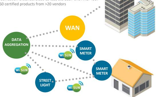
FAN: Communication Between Smart Meters and Distribution Automation
