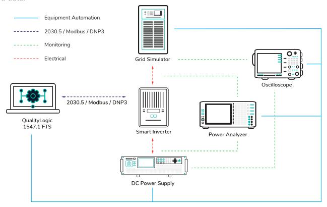
**DER Protocols** – Supports the 2030.5, SunSpec Modbus, and DNP3 communications required by each of the IEEE 1547.1 Interoperability tests with the target DER.
