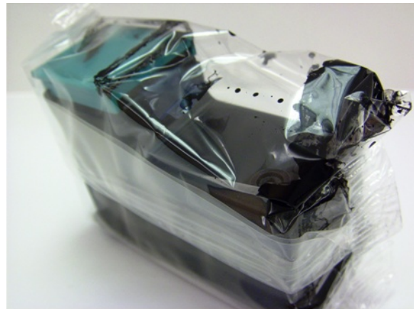
Refill Station brand cartridge leaking ink into the shipping container.
