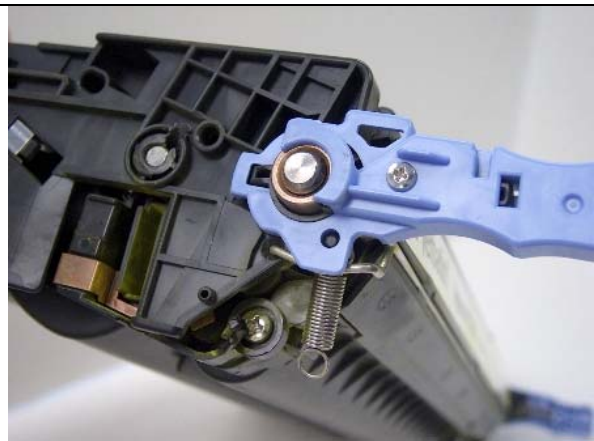
Brand E yellow cartridge with a broken wiper door spring. No pages could be printed.
